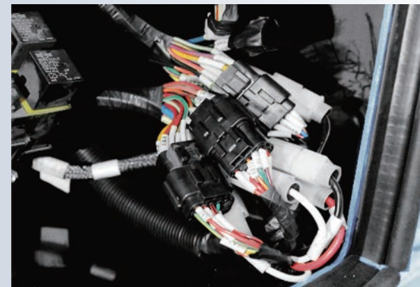
Dust proof and water proof sockets and plugs: protection degree IP65
