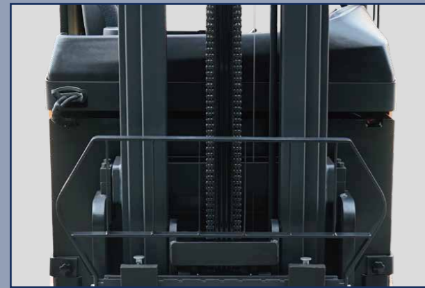
■ Optimal mast width and hose lay-behind ensure a clear view through the mast.
